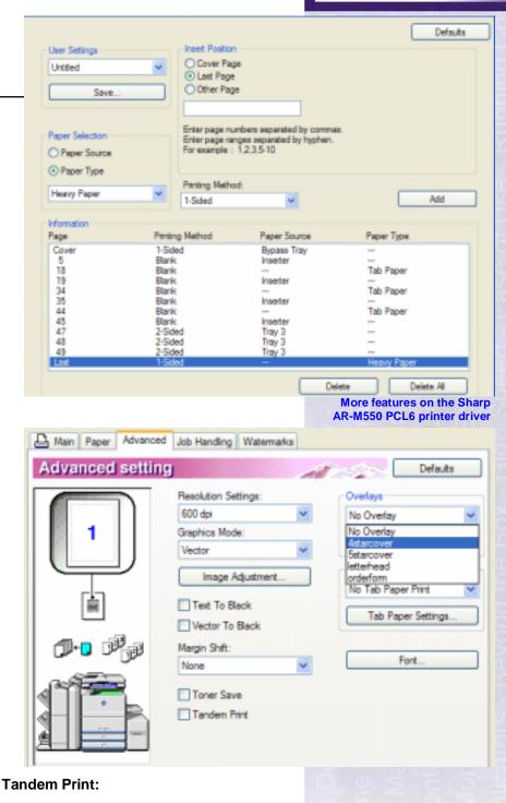
Sharp includes tandem printing within its standard print function (obviously requiring two print-enabled devices). The job is sent to the master tandem device, which splits the job and sends the data file to the slave tandem device with instruction on how many sets to reproduce.
